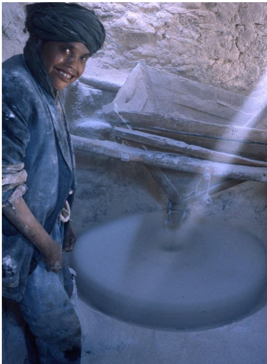
The rushing water drives a horizontal grinding wheel. The air is filled with flour dust. Ingenuity at its finest.
